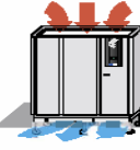
Downflow unit with discharge from the front. Downflow unit with floor stand.
