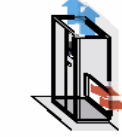
Upflow unit with discharge from the base. Upflow unit with manifold air filter.
