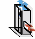
Upflow unit with discharge from the rear. Upflow unit with manifold air filter.
