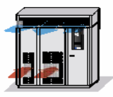
Upflow unit with discharge on the top. Upflow unit with manifold air filter.
