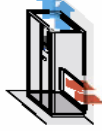
Upflow unit with suction from the rear Downflow unit with discharge from the top
