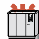
Downflow unit with suction from the front and discharge on the top Downflow unit with suction from the front
