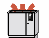
Downflow unit with suction from the front and discharge from the top Downflow unit with suction from the front
