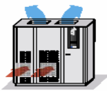
Upflow unit with discharge on the top Downflow unit with suction from the side
