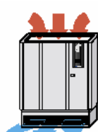
Downflow unit with enhanced rear and front discharge. Uniti Downflow con scarico di mandata frontale.
