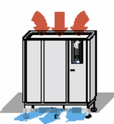
Downflow unit installed on floor stand. Uniti Downflow installati su piedistallo regolabile.
