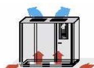
Uniflair unit with suction from the base. Uniflair unit with suction from the base.
