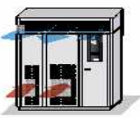
Uniflair unit with discharge plenum. Uniflair unit with discharge plenum.
