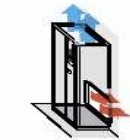
Uniflair unit with suction from the side. Uniflair unit with suction from the side.
