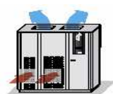
Uniflair unit with discharge on the side. Uniflair unit with discharge on the side.
