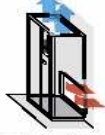
Upflow unit with air suction from the base and hot gas reheat on the side.
