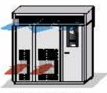
Upflow unit with air discharge on the top and hot gas reheat on the side.
