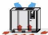
Upflow unit with air suction from the base and hot gas reheat on the side.
