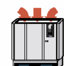
Downflow unit with hot water reheat on the top and hot gas reheat on the side.
