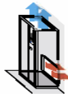
Upflow unit with suction from the rear. Downflow unit with discharge on the top.
