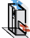
Upflow unit with suction from the rear. Downflow unit with discharge on the top.
