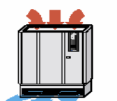
Downflow unit with suction from the front and discharge on the top. Downflow unit with suction from the front.
